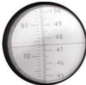
Figure 2. Refractive index values as read on the scale
